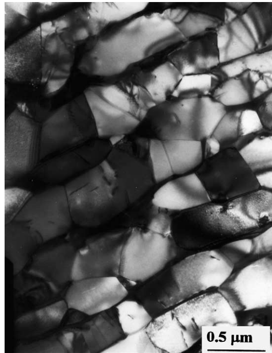
Fig. 2. Bright field image of the Zr–2.5Nb in the as-received condition. The micrograph clearly shows the \beta phase at the \alpha/\alpha grain boundaries.
